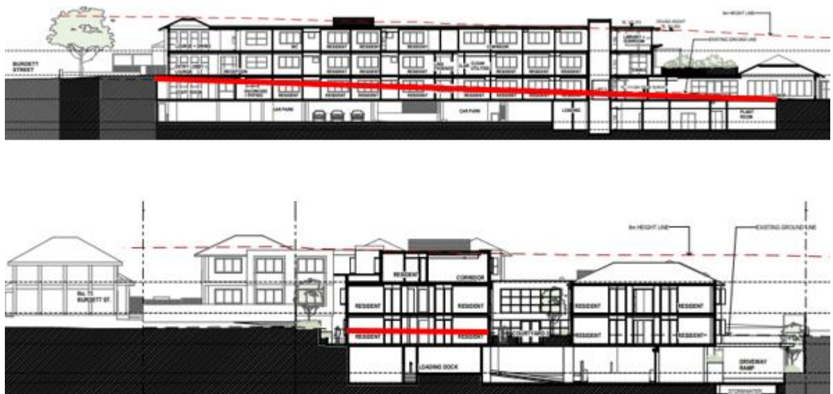
Figure 2 – Section showing the 3 storey elements located through the central portion of the eastern building pavillion with the red line representing existing ground level
