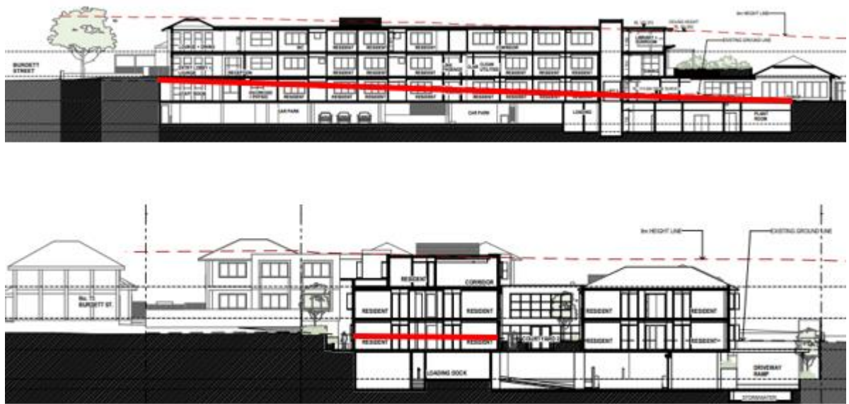
Figure 1 – Section showing the 3 storey elements located through the central portion of the eastern pavilion with the red line representing existing ground level
